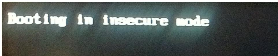
The fact that the system is booting in insecure mode means it has failed to verify the boot loader because we have not enrolled the key yet. Once we include the key in UEFI, the firmware system will not show this Message.
