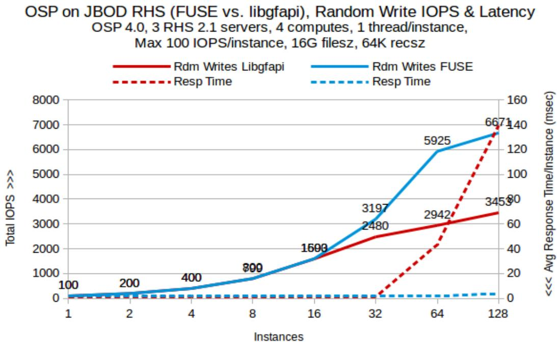
Figure 4.15: FUSE vs. Libgfapi - Random Write IOPS & Latency
