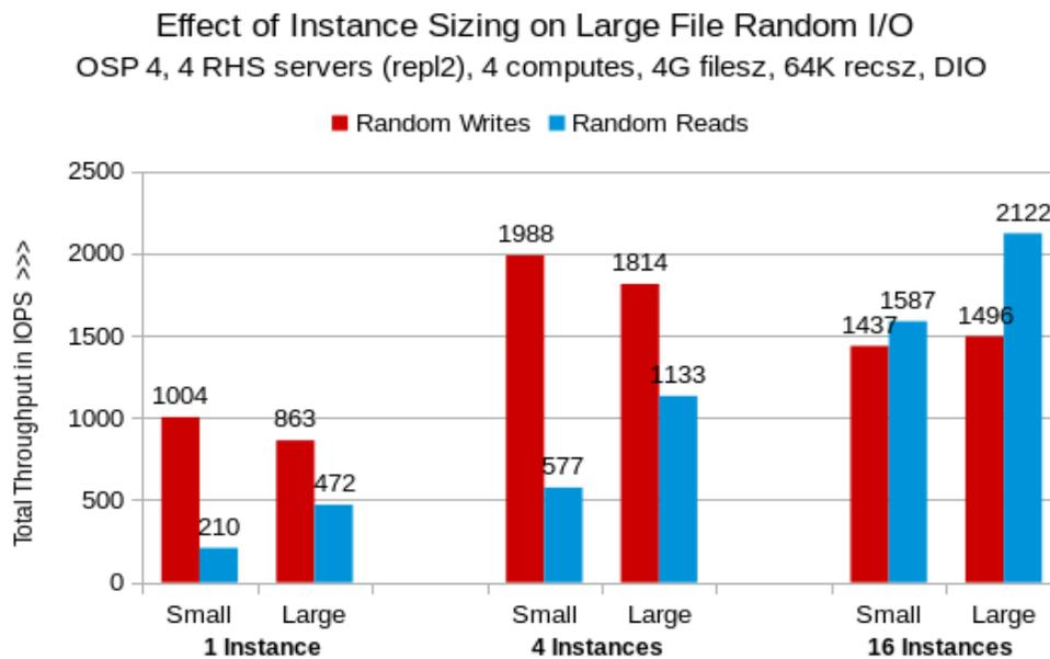
Figure 5.3: Effect of Instance Size on Large File Random I/O
