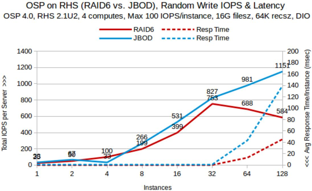
Figure 4.11: RAID6 vs. JBOD - Random Write IOPS & Latency
