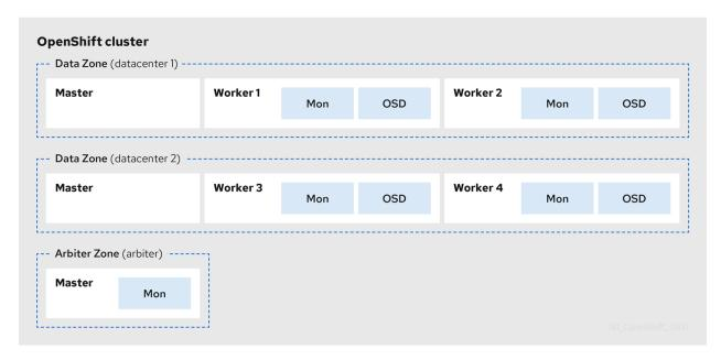
In the diagram the OpenShift Data Foundation monitor pod deployed in the Arbiter zone has a built-in tolerance for the master nodes. The diagram shows the master nodes in each Data Zone which are required for a highly available OpenShift Container Platform control plane. Also, it is important that the OpenShift Container Platform nodes in one of the zones have network connectivity with the OpenShift Container Platform nodes in the other two zones.
