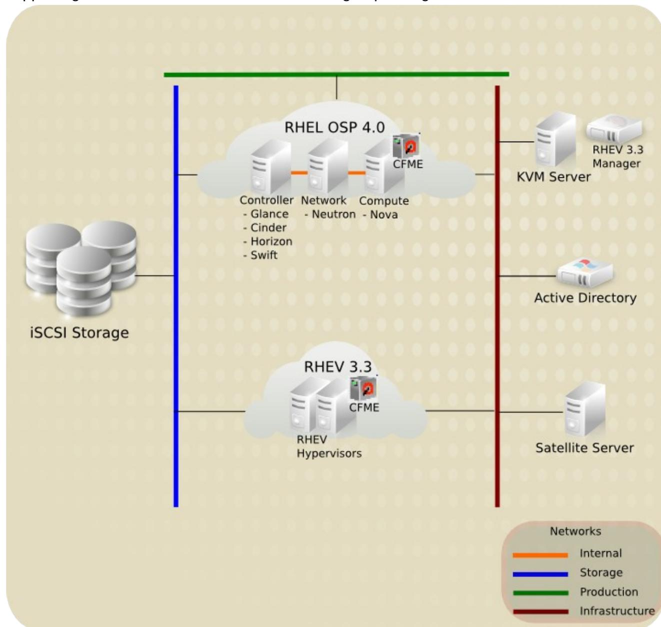
Figure 3-1: Reference Architecture Components
