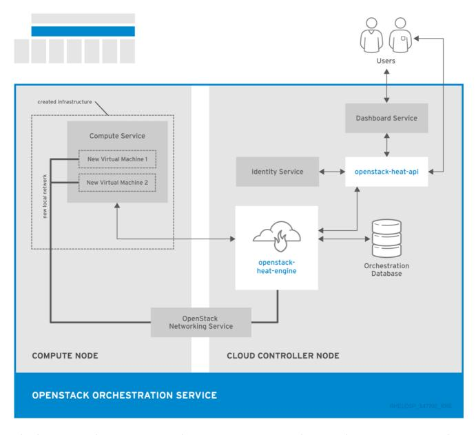
The director uses the native OpenStack Heat APIs to provision and manage the resources associated with deploying an Overcloud. This includes precise details such as defining the number of nodes to provision per node role, the software components to configure for each node, and the order in which the director configures these components and node types. The director also uses Heat for troubleshooting a deployment and making changes post-deployment with ease.
