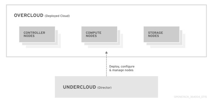
Director ships with tools, utilities, and example templates for creating an Overcloud configuration. The director captures configuration data, parameters, and network topology information then uses this information in conjunction with components such as Ironic, Heat, and Puppet to orchestrate an Overcloud installation.
