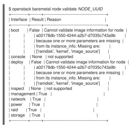
Replace *NODE\_UUID* with the unique identifier for the node. Alternatively, use the node's logical name. The output of the command above should report either **True** or **None** for each interface. Interfaces marked **None** are those that you have not configured, or those that are not supported for your driver.
