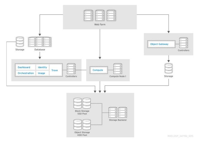
In this example, Ceph provides a Swift-compatible REST interface, as well as block-level storage from a distributed storage cluster. It is highly flexible and enables reduced cost of operations with features such as self-healing and auto-balancing. Erasure coded pools are recommended to maximize the amount of usable space.
