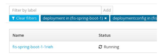
9. Click on the pod **Name** (in this example, **fis-spring-boot-1-1rieh**) to view the details of the running pod.
