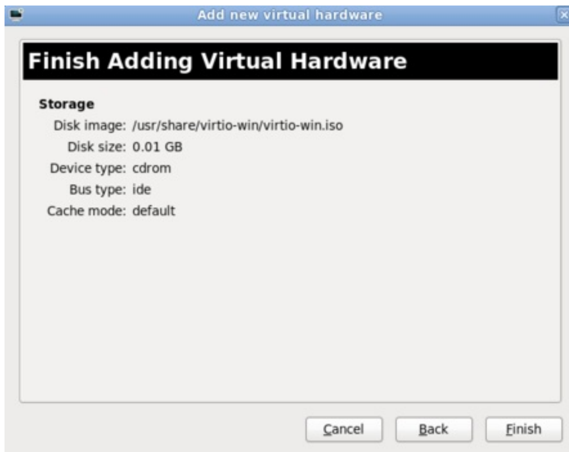
Figure 10.4. The Add new virtual hardware wizard in Red Hat Enterprise Linux 6.1
