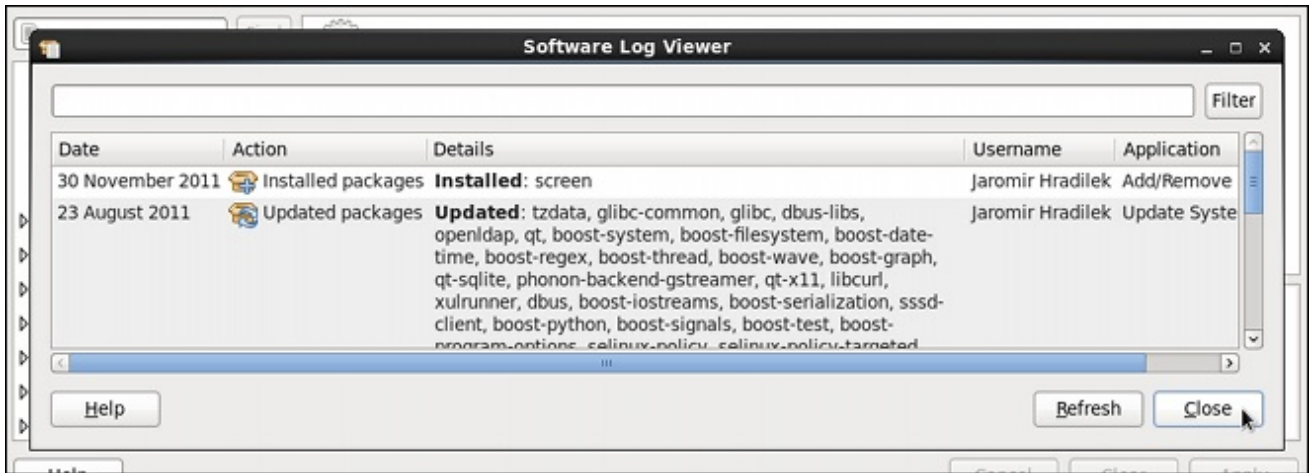
Figure 9.10. Viewing the log of package management transactions with the Software Log Viewer
