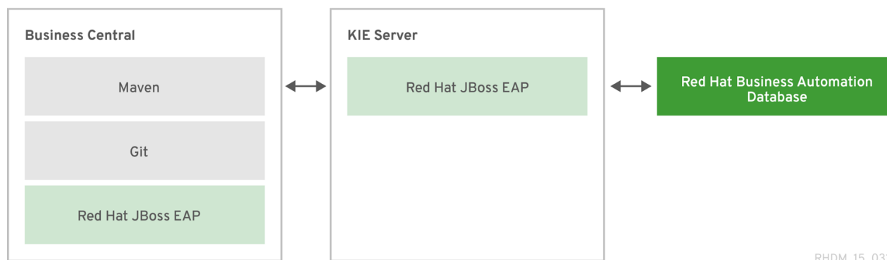
Figure 6.2. Red Hat Decision Manager on Red Hat JBoss EAP with Business Central and Decision Server
