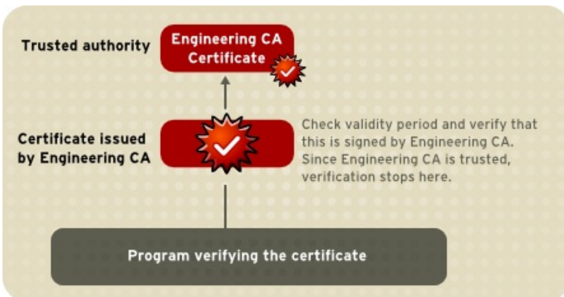
Figure 1.9. Verifying a Certificate Chain to an Intermediate CA
