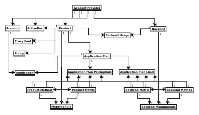
The 3scale operator provides custom resource definitions and their relations, which are visible in the following diagram.
