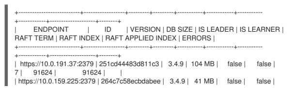
This example shows that the database size for this etcd member is now 41 MB as opposed to the starting size of 104 MB.
