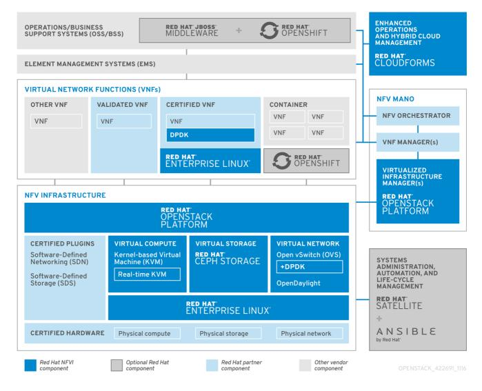
In general, a network functions virtualization (NFV) platform has the following components:
