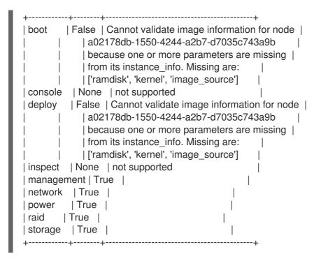
Replace *NODE\_UUID* with the unique identifier for the node. Alternatively, use the node's logical name. The output of the **openstack baremetal node validate** command should report either **True** or **None** for each interface. Interfaces marked **None** are those that you have not configured, or those that are not supported for your driver.
