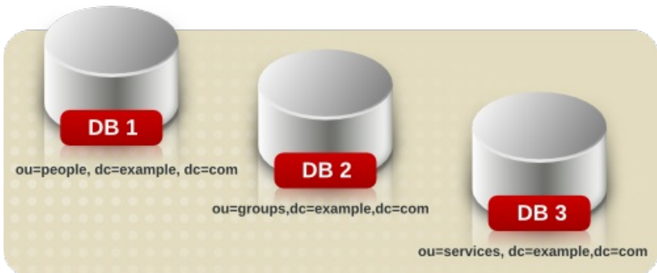
Figure 6.1. Storing Suffix Data in Separate Databases
