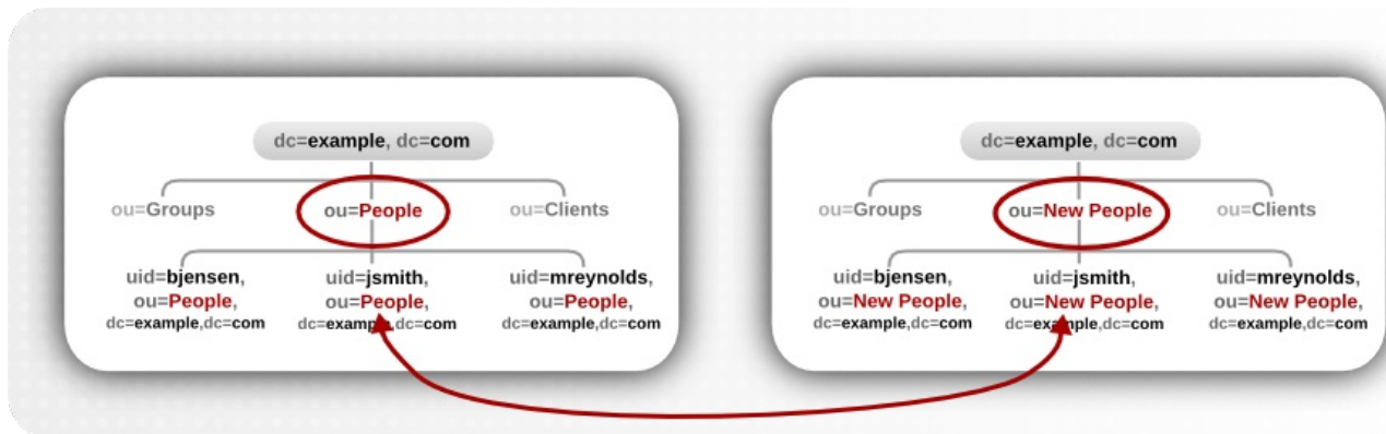
Figure 4.11. modrdn Operations for a Subtree Entry
