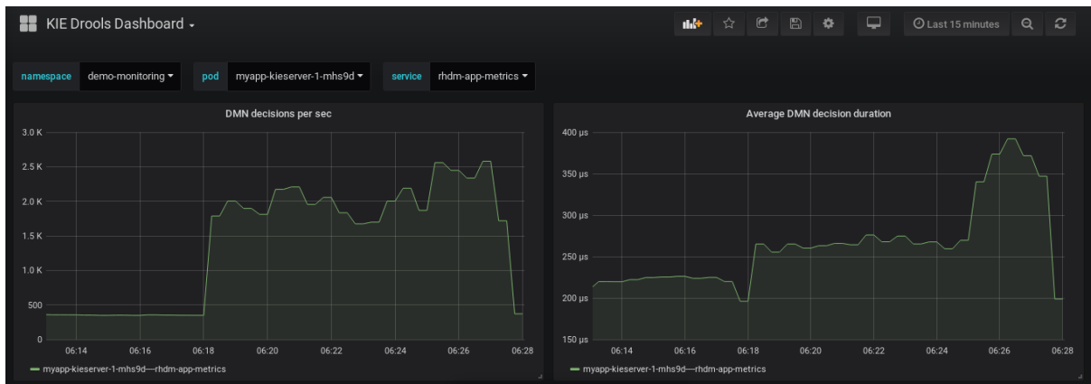
Figure 16.3. Grafana dashboard with KIE Server metrics for DMN models
