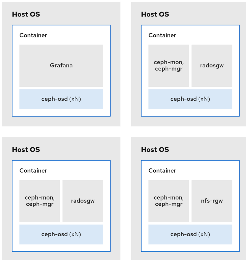
Figure 2.4. Colocated Daemons Example 3
