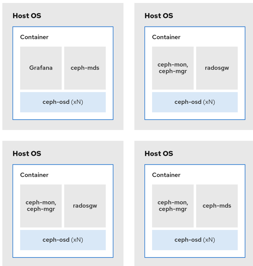
Figure 2.3. Colocated Daemons Example 2
