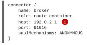
If the broker is running in the same OpenShift cluster as the router mesh, then use the service IP address. If the broker is running in a different OpenShift cluster, then use the fully-qualified domain name of that OpenShift cluster's route.
