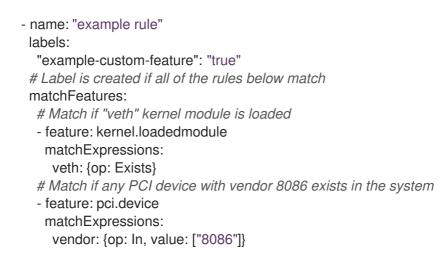
This custom resource specifies that labelling occurs when the **veth** module is loaded and any PCI device with vendor code **8086** exists in the cluster.
