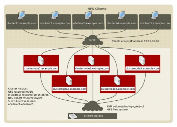
Figure 2.1. NFS over GFS in a 5-Node Cluster
