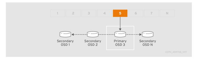
When the primary OSD fails and gets marked out of the cluster, CRUSH assigns the placement group to another OSD, which receives copies of objects in the placement group. Another OSD in the **Up Set** will assume the role of the primary OSD.
