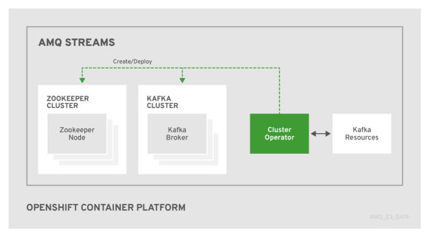
When the Cluster Operator is up, it starts to *watch* for certain OpenShift resources containing the desired Kafka, Kafka Connect, or Kafka Mirror Maker cluster configuration. By default, it watches only in the same namespace or project where it is installed. The Cluster Operator can be configured to watch for more OpenShift projects or Kubernetes namespaces. Cluster Operator watches the following resources:
