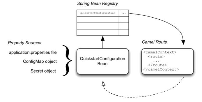
The configuration mechanism has the following main parts:
