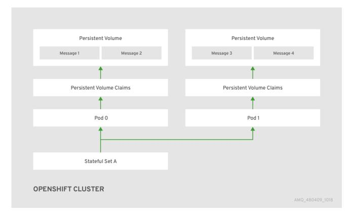
When you take a broker pod offline, the StatefulSet is scaled down and you must manage what happens to the message data in the unattached PV. To migrate the messages held in the PV associated with the now-offline pod, you use the scaledown controller. The process of migrating message data in this fashion is sometimes referred to as *pod draining*.
