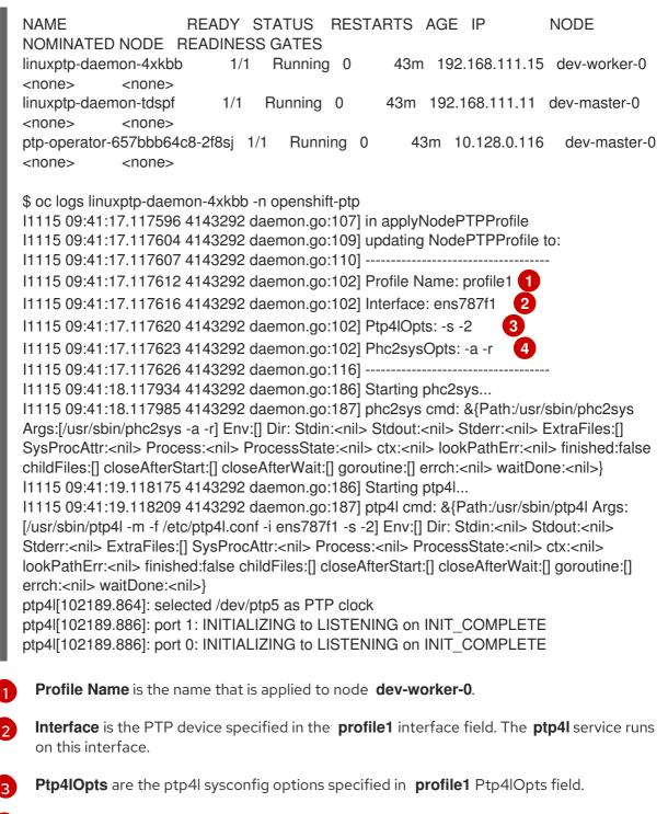
Phc2sysOpts are the phc2sys sysconfig options specified in profile1 Phc2sysOpts field.
