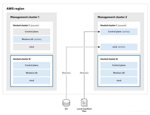
4. The external DNS API is accessible again, and the worker nodes use it to move to management cluster 2. The external DNS API can access the load balancer that points to the control plane.
