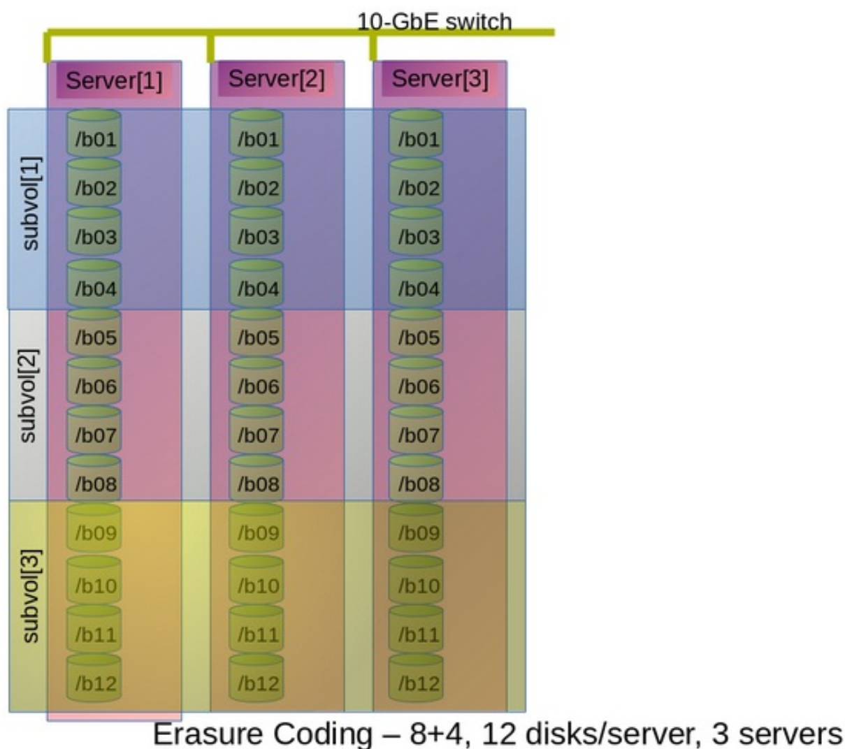
Figure 11.1. Example Configuration of 8+4 Dispersed Volume Configuration
