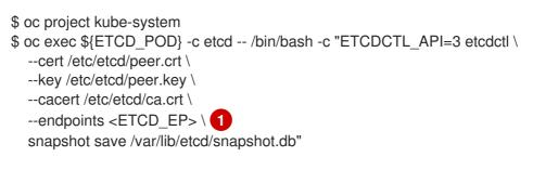
Specify the etcd endpoint IP address that you obtained.
