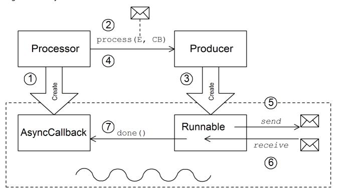
The asynchronous producer processes an exchange as follows:
