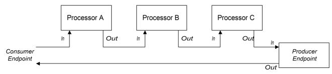
Note that in order to support the **InOut** exchange pattern, it is **essential** that the last node in the route (whether it is a producer endpoint or some other kind of processor) creates an **Out** message. Otherwise, any client that connects to the consumer endpoint would hang and wait indefinitely for a reply message. You should be aware that not all producer endpoints create **Out** messages.
