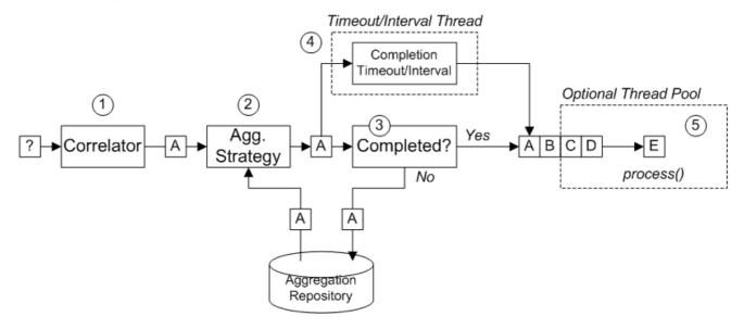
The incoming stream of exchanges shown in Figure 8.6, "Aggregator Implementation" is processed as follows:
