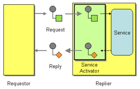
In many respects, a service activator resembles a conventional remote procedure call (RPC), where operation invocations are encoded as messages. The main difference is that a service activator needs to be more flexible. An RPC framework standardizes the request and reply message encodings (for example, Web service operations are encoded as SOAP messages), whereas a service activator typically needs to improvise the mapping between the messaging system and the service's operations.
