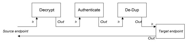
The pipeline connects the output of each endpoint to the input of the next endpoint. The **Out** message from the final endpoint is sent back to the original caller. You can define a route for this pipeline, as follows:
