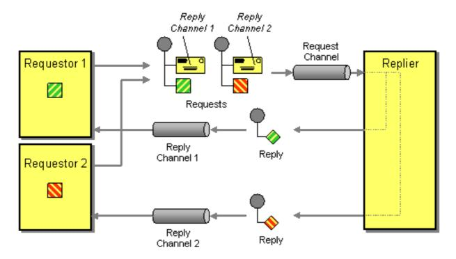
For example when using JMS with **InOut**, the component will by default be returned to the address given in **JMSReplyTo**.
