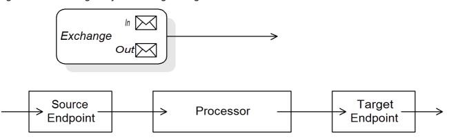
Figure 34.1, "Exchange Object Passing through a Route" shows an exchange object passing through a route. In the context of a route, an exchange object gets passed as the argument of the **Processor.process()** method. This means that the exchange object is directly accessible to the source endpoint, the target endpoint, and all of the processors in between.
