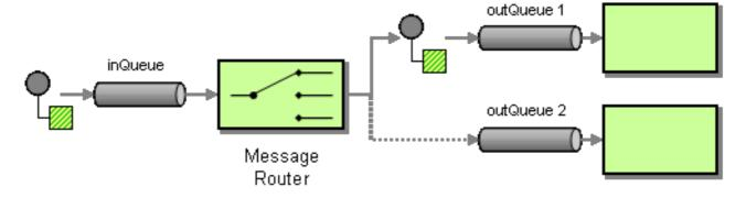
A message router can easily be implemented in Apache Camel using the **choice()** processor, where each of the alternative target endpoints can be selected using a **when()** subclause (for details of the choice processor, see Section 1.5, "Processors").
