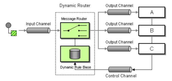
In **Camel 2.5** we introduced a **dynamicRouter** in the DSL, which is like a dynamic Section 8.7, "Routing Slip" that evaluates the slip **on-the-fly**.
