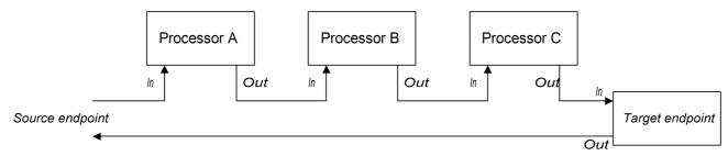
The processors in the pipeline look like services, where the **In** message is analogous to a request, and the **Out** message is analogous to a reply. In fact, in a realistic pipeline, the nodes in the pipeline are often implemented by Web service endpoints, such as the CXF component.
