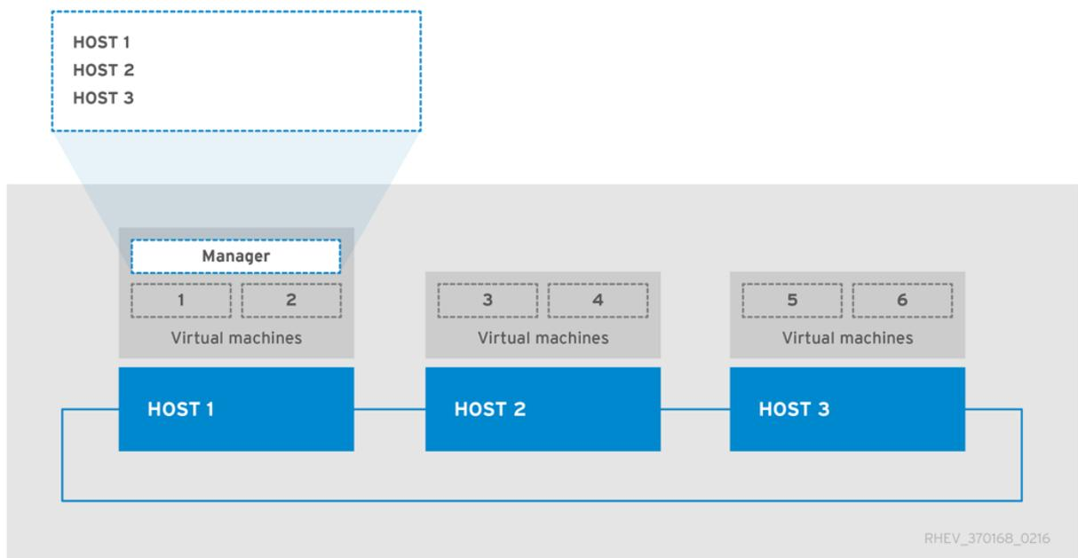
**Host 2** and **Host 3** have been re-deployed into the restored environment. The environment is now as it was in the first image, before the backup was taken, with the exception that the Manager virtual machine is hosted on **Host 1**.
