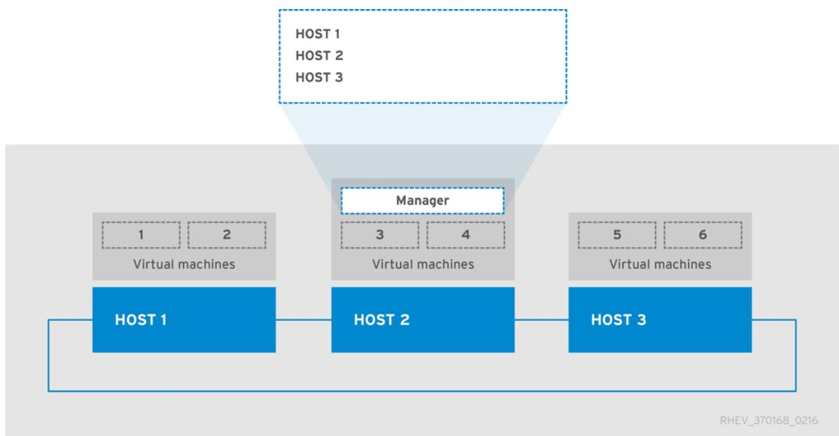
Place **Host 1** into maintenance mode. This will migrate the virtual machines on **Host 1** to the other hosts, freeing it of any virtual load and enabling it to be used as a failover host for the backup.
