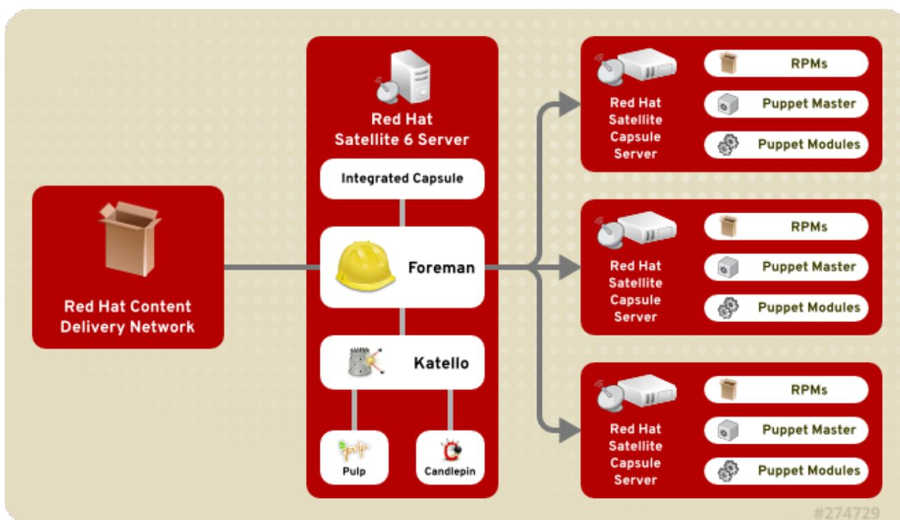
Figure 1.1. Red Hat Satellite 6 System Architecture
