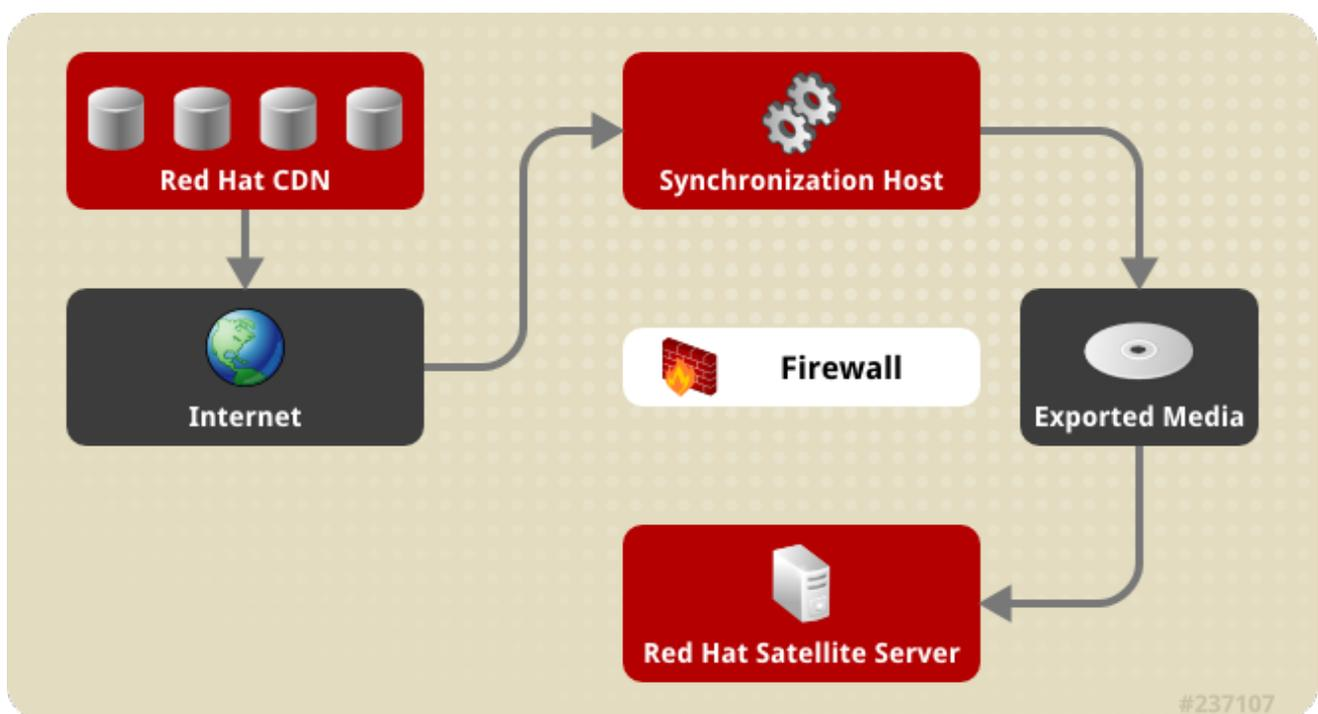
Figure 4.1. Disconnected Satellite
