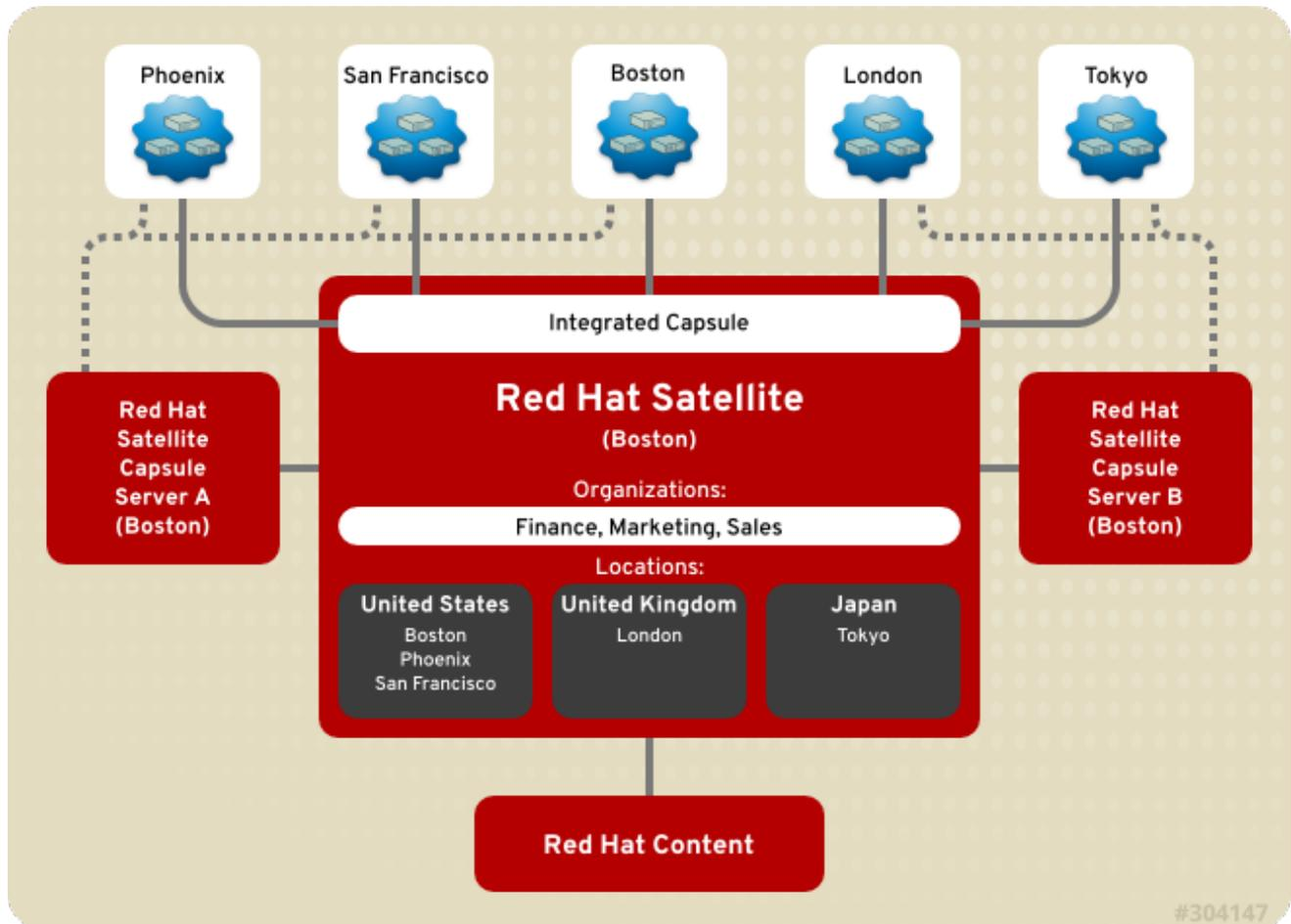
**Figure 1.3. Single Satellite with Integrated Capsule and Backup Capsules**
