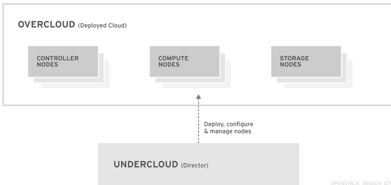
Director ships with tools, utilities, and example templates for creating an Overcloud configuration. The director captures configuration data, parameters, and network topology information then uses this information in conjunction with components such as Ironic, Heat, and Puppet to orchestrate an Overcloud installation.
