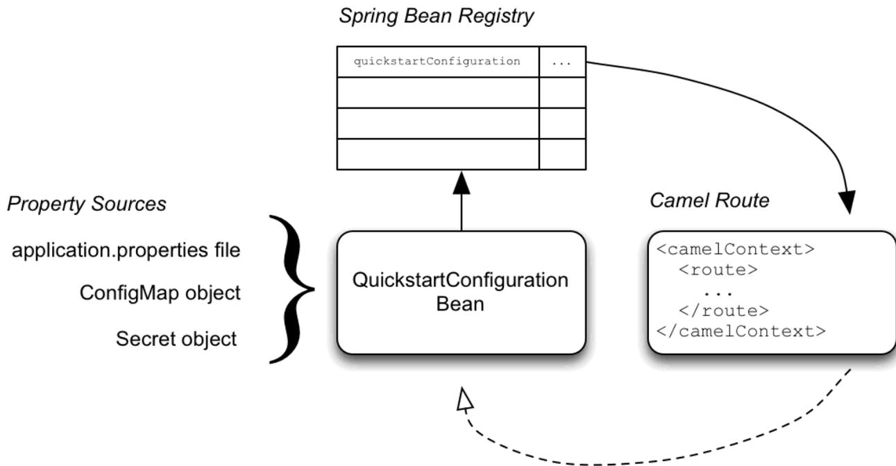
The configuration mechanism has the following main parts:
