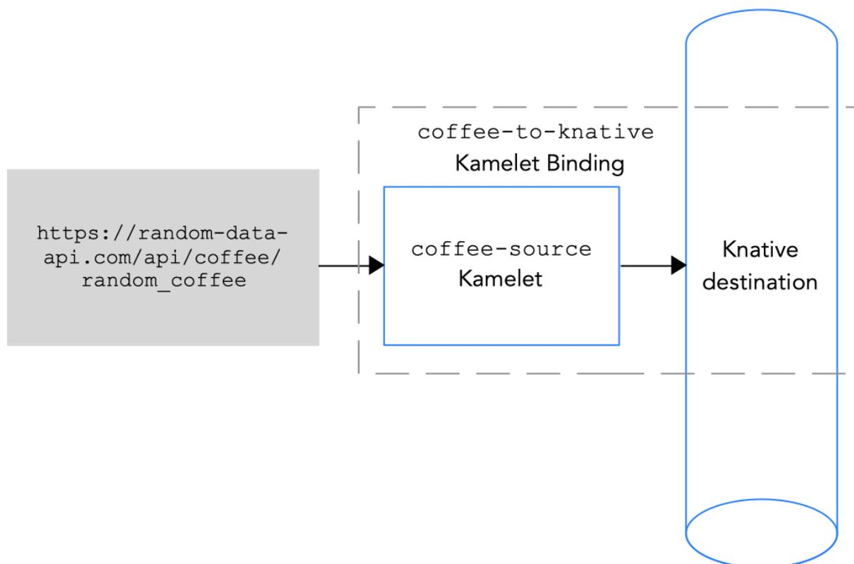
**Figure 3.2** Connecting a data source to a Knative destination
