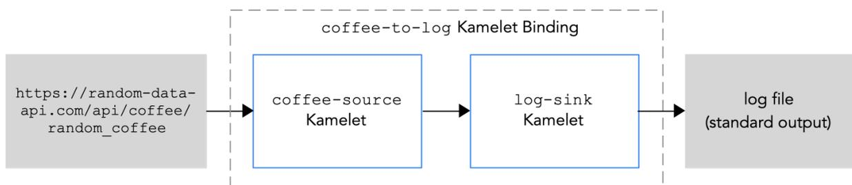
Figure 1.2: Example Kamelet Binding
