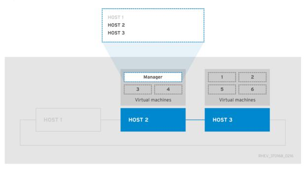
Use **engine-backup** to create backups of the environment. After the backup has been taken, **Host 1** can be activated again to host virtual machines, including the engine virtual machine.
