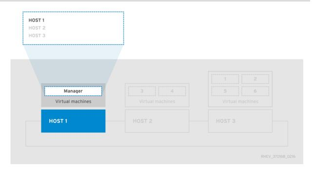
After **Host 1** and the engine virtual machine have synchronized and the deployment has been finalized, the environment can be considered operational on a basic level. With only one hosted-engine host, the engine virtual machine is not highly available. However, if necessary, high-priority virtual machines can be started on **Host 1**.
