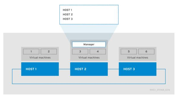
Place **Host 1** into maintenance mode. This will migrate the virtual machines on **Host 1** to the other hosts, freeing it of any virtual load and enabling it to be used as a failover host for the backup.
