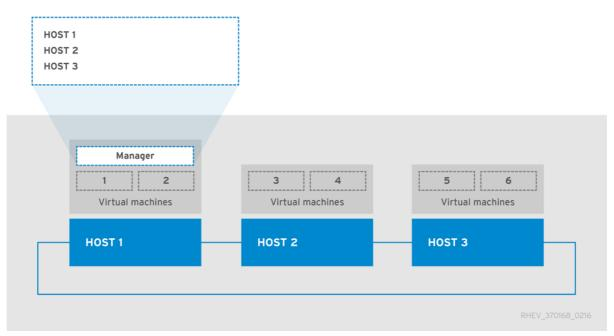
**Host 2** and **Host 3** have been re-deployed into the restored environment. The environment is now as it was in the first image, before the backup was taken, with the exception that the engine virtual machine is hosted on **Host 1**.
