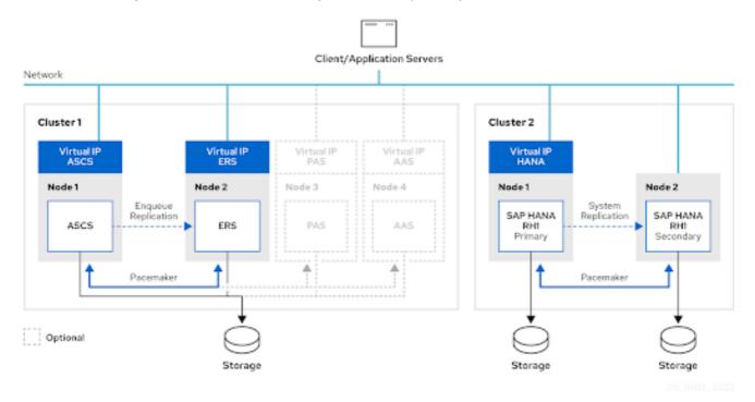
Even though the diagram shows that it is optionally possible to also have Primary and Additional Application Server (PAS/AAS) instances managed on separate servers, it is also supported to have these instances running on the same HA cluster nodes as the **(A)SCS** and **ERS** instances and have them managed by the cluster.
