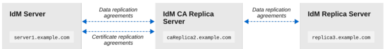
Figure 8.1. Replication Topology used in this example
