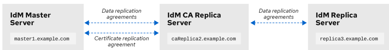
Figure 7.1. Replication Topology used in this example
