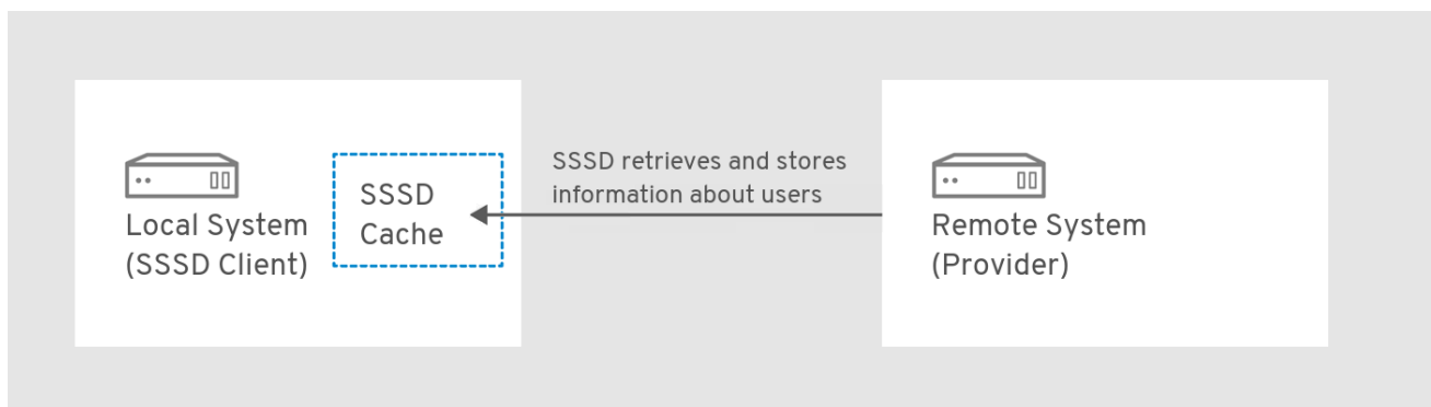
Figure 2.1. How SSSD works
