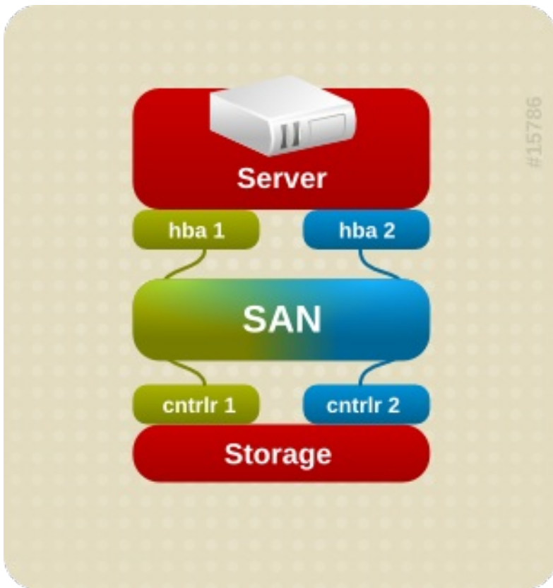
Figure 1.3. Active/Active Multipath Configuration with One RAID Device
