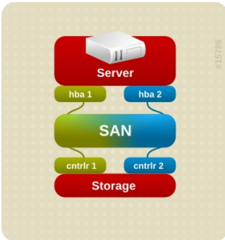
Figure 1.3. Active/Active Multipath Configuration with One RAID Device
