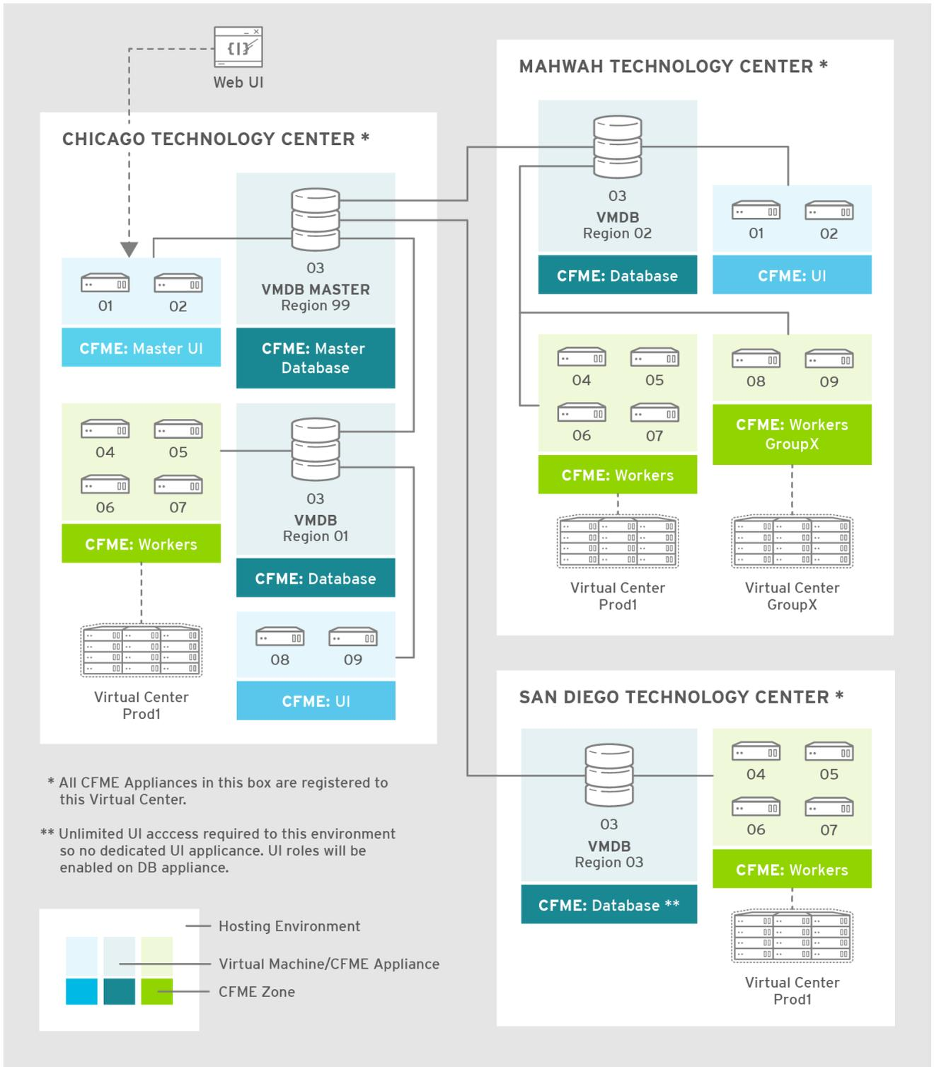
The Master appliance is located in Chicago and contains a master region and a subregion that manages the worker appliances. The Mahwah technology center contains a single subregion that manages two zones. Likewise, the San Diego technology center contains a single subregion managing a single zone.
