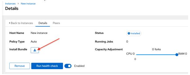
The install bundle contains TLS certificates and keys, a certificate authority, and a proper Receptor configuration file.
