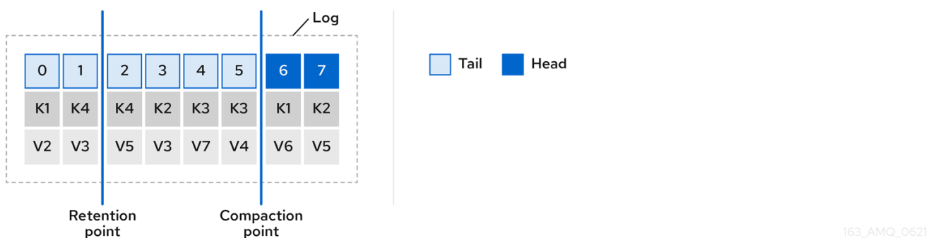
Figure 13.3. Log retention point and compaction point
