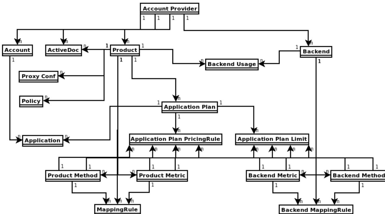
The 3scale operator provides custom resource definitions and their relations, which are visible in the following diagram.
