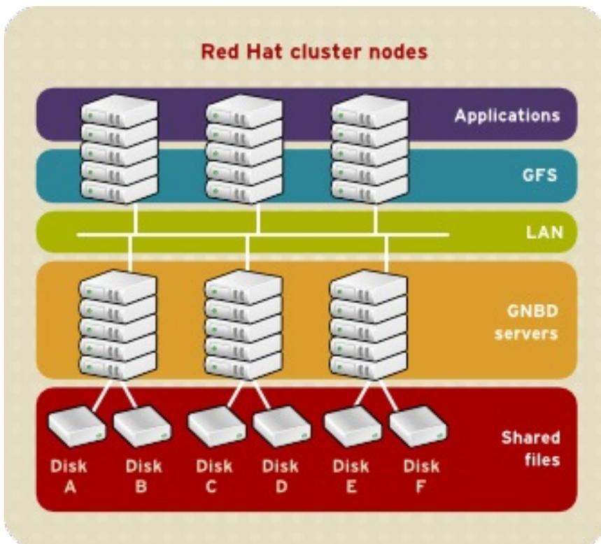
Figure 2.3. GFS and GNBD with Directly Connected Storage
