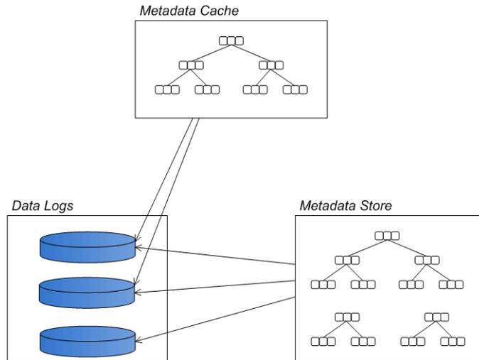
Messages are stored in file-based data logs. When all of the messages in a data log have been successfully consumed, the data log is marked as deletable. At a predetermined clean-up interval, logs marked as deletable are either removed from the system or moved to an archive.
