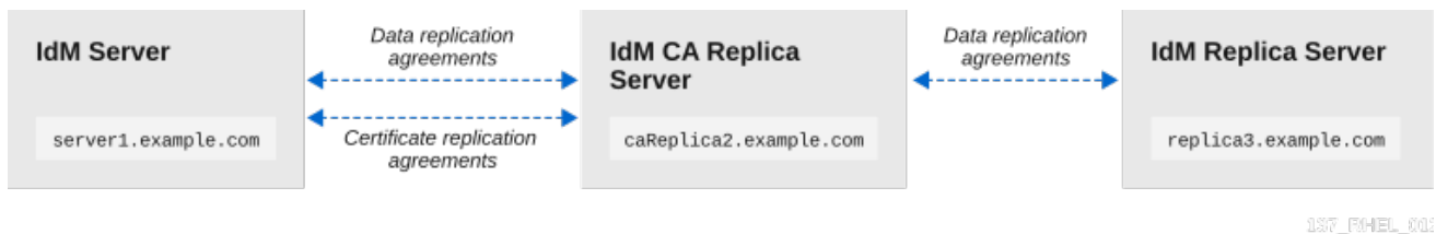
Figure 5.1. Replication Topology used in this example
