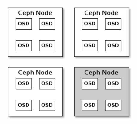
In a typical production Ceph cluster, a Ceph OSD node has a particular hardware configuration that facilitates a particular type of storage strategy. Since a Ceph OSD node is part of a CRUSH hierarchy, the performance impact of adding or removing a node typically affects the performance of pools that use that CRUSH hierarchy (i.e., CRUSH ruleset).
